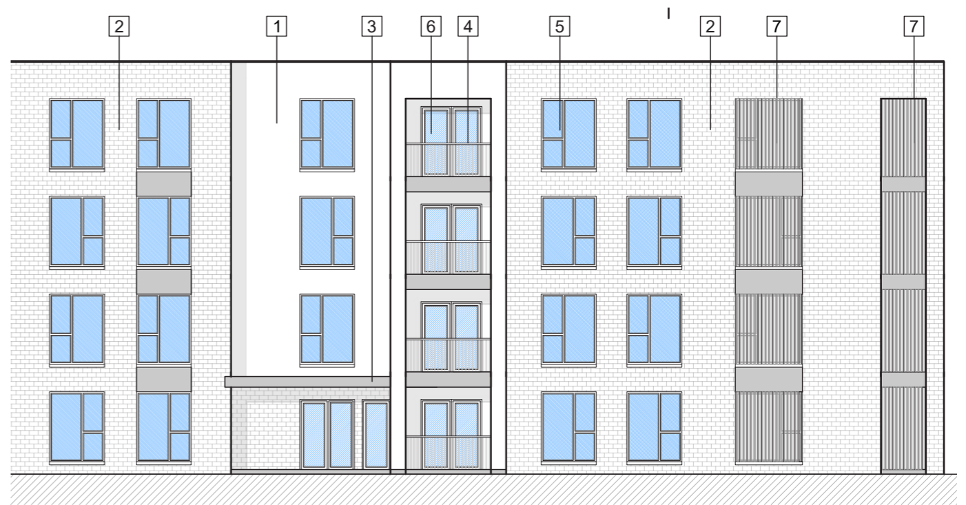
Apartment Block J Louvre System on Eastern Elevation
